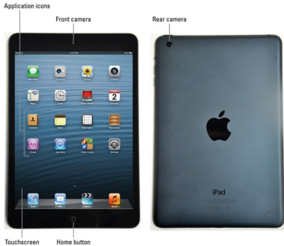
Figure 1-4: The front and back of the iPad mini is a study in elegant simplicity.
