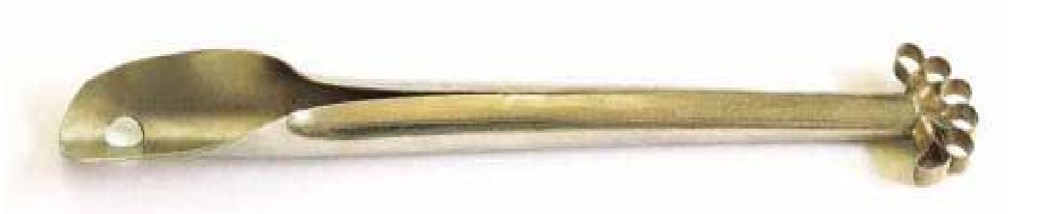
COCONUT SCRAPER (PANGKAYOD) Made of iron or steel to scrape coconut applied as the coco direction and in on scraper produces s finer strips, use the holes. The coconut s the flesh of various n
