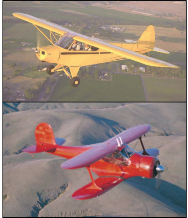
Figure 1-5. Monoplane and biplane.
