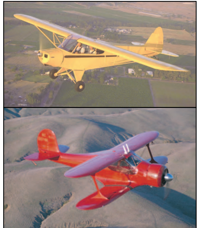
Figure 1-5. Monoplane and biplane.
