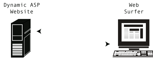
Figure 1-7. Illustration of how data is exchanged between a dynamic site and the web surfer
