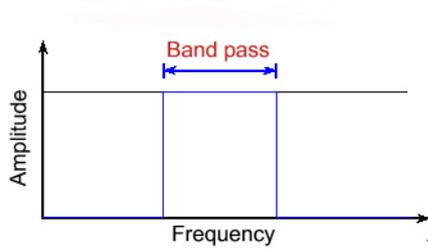
A filter that passes frequencies between two limits is known as a **band-pass filter**.
