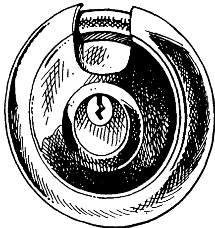
Figure 9. Mushroom and spool pin padlock.
